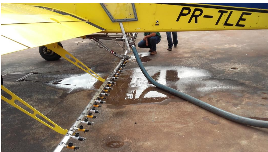
Figura 2. Aeronave Air Tractor502 equipada com bicos STOL ULD.
